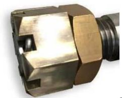
For decades there has been a nut available that is specifically designed to be held in place with a cotter pin. It is called a castle nut or castellated nut. In most cases these nuts have to be custom made in a machine shop for each propeller and shaft setup for everything to line up correctly due to the limited depth of the notches.
